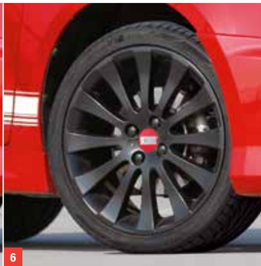
6 | Alloy rim "X-ITE" 7 J x 17" matt black 12-spoke design, suitable for 205/40 R17, incl. screws, matt black wheel bolt covers and ablaze red pearl metallic centre cap with silver X-ITE logo, for two wheel drive only
