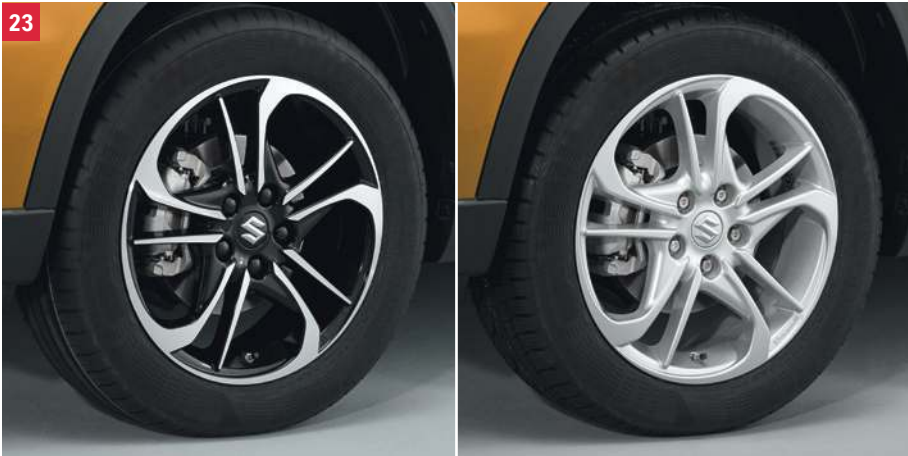
23 | ALLOY RIM "MOJAVE" 6,5 J x 17" suitable for 215/55 R17 tyres, including centre cap with Suzuki logo, ECE-R 124 approval. Black polished Part No. 43210-54PU0-0SP Silver Part No. 43210-54PS0-0KS
