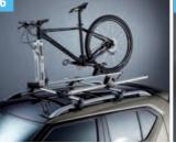
For transporting bicycles without front wheel (one set for one bike). Maximum roof load is 30kg for models without roof rail and 50kg for those with roof rail. Only in combination with multi roof rack 78901-62R20-000 or 78901-62R30-000. Own weight: 2.5kg
