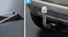
The maximum towing capacity 1,000kg and the maximum vertical load 50kg. Part No. 72901-62R01-000
