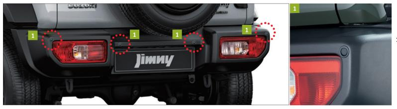
1 | REAR PARKING SENSORS Set of four paintable sensors and piezo buzzer.
