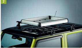
1 | MULTI ROOF RACK<sup>1,2</sup> Black rectangular profile steel with end caps. Own weight: 6.3 kg Dimensions: 70 cm × 144.4 cm × 18.3 cm
