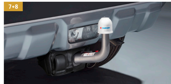
7 | Tow Bar 1 Detachable, for trailers and carrier systems. The max vertical load : 75kg The max towing capacity : 1,500kg Part No. 9927D-86R00-000
