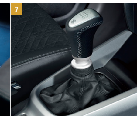
7 | Gear Shift Knob 48V Suitable for LHD and RHD, with silver inlay and silver stitching. For 6M/T. Part No. 990E0-61M37-000
