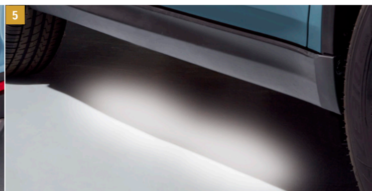
5 | LED Coming Home Function Upon opening front doors, the area below the front doors of the vehicle is illuminated to assist passengers to find their way. Part No. 99000-990B4-132
