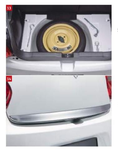
13 | Spare Tire Set<sup>1</sup> WVTA • Includes spare tire kit, fixation kit, jack, jack bracket kit, spare tire under sheet, and wrench.
